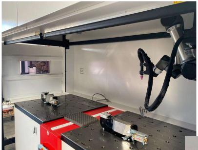
Air intakes which act as a predisposition for pneumatic jigs and masks
