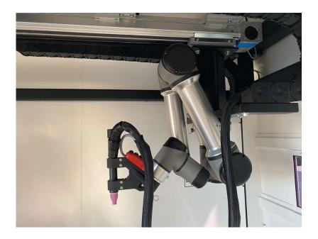
Implemented linear guide seventh axis by Festo, allows the robot to move among working tables
